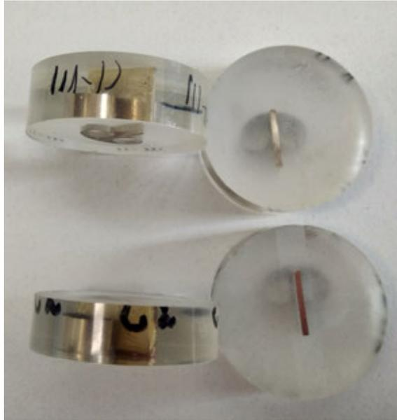
**Figure 16** – Exemplary picture of fire gilded copper and silver substrates embedded in epoxyresin and subsequently cut and polished for cross section analysis. Top: Silver substrate; Bottom: Copper substrate
