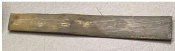
**Figure 14** – Picture of a temperature gradient sample (cg). The sample was heated from the left side.
