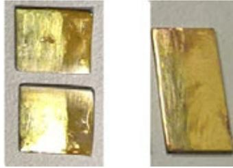
**Figure 13** – Fire gilded silver (left) and copper (right) sheets. The left side of each sample is polished.
