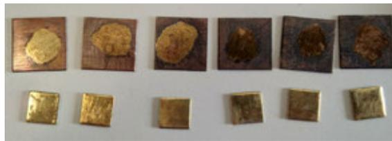
**Figure 15** – Exemplary picture of a series of artificial aging samples. Artificial aging time increases from left to right. Copper substrates at the top, silver substrates at the bottom. The samples were treated with 200°C between 0.25 (left) and 21 (right) days, more details can be found in table 8 for samples Cu/Ag I-x.
