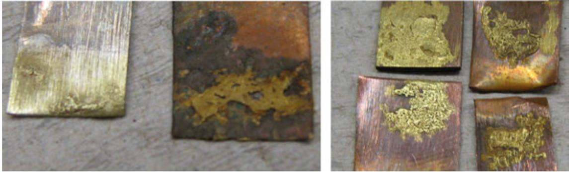
**Figure 12** – Pictures of fire gilding done wrong, showcasing some common difficulties and mistakes. Left: Heating for too long. The golden color fades out on the silver substrate due to diffusion, and the golden layer crumbling off the copper substrate due to oxidation. Right: Irregular golden layer on copper substrates due to insufficiently adherent amalgam before heating. [15].
