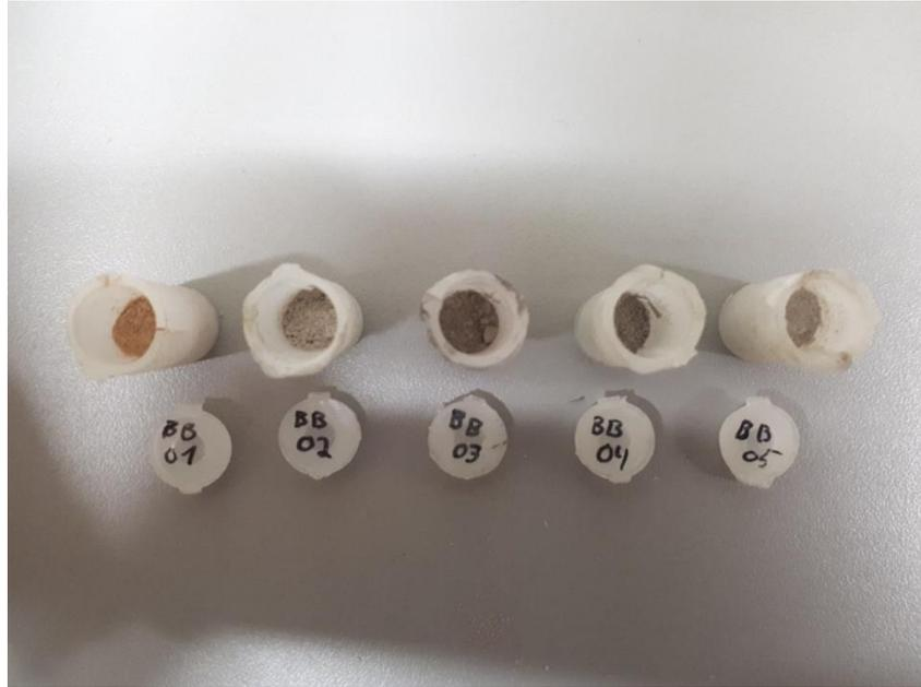
**Figure 10:** Heavy concrete samples in their powder form.
